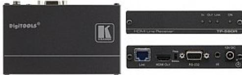
The TP-580R is a 4K UHD, twisted pair receiver for HDMI, bidirectional RS-232 and IR signals. It supports resolutions up to 4K@60 UHD (4:2:0). The TP-580T converts HDMI, RS-232, and IR signals into a twisted pair signal that it transmits to a TP-580R receiver. The TP-580R converts the twisted pair signal back into HDMI, bidirectional RS-232 and IR signals
